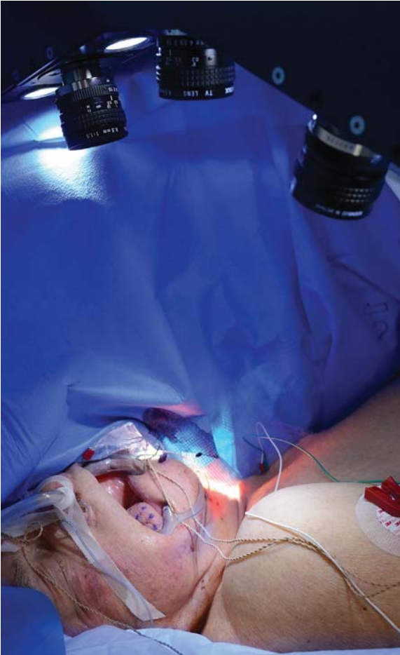
Figure 5.2 | Surgical drape separates the non-sterile environment from the operation field. The triple-camera setup is positioned in front of the mouth opening. The tongue markers are made visible by a lip retractor.
